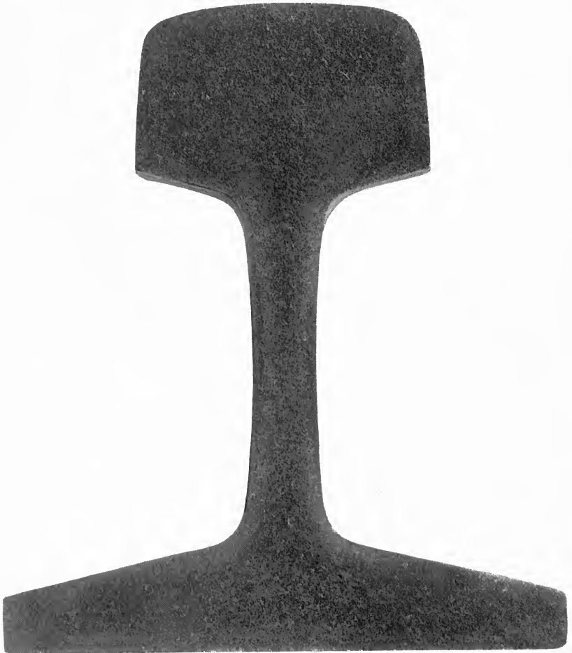
VANADIUM STEEL HEAT 27989, RAIL "A" Shows a perfectly uniform, dense structure with no evidence of residual piping.
